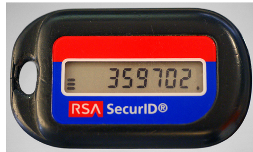
Figure 1 - example of an OTP token (RSA SecurID)
