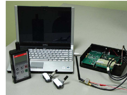
Figure 2: Equipment used for packet sniffing. At the bottom, from left to right are the ATEQ VT55 TPMS trigger tool, two tire pressure sensors (TPS-A and TPS-B), and a low noise amplifier (LNA). At the top is one laptop connected with a USRP with a TVRX daughterboard attached.
