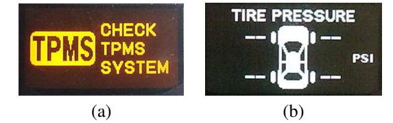
Figure 16: Dash panel snapshots indicating the TPMS system error (this error cannot be reset without the help of a dealership): (a) the vehicle’s general-information warning light; (b) tire pressure readings are no longer displayed as a result of system function errors.
