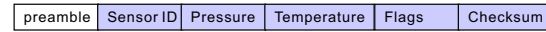
Figure 4: An illustration of a packet format. Note the size is not proportional to real packet fields.
