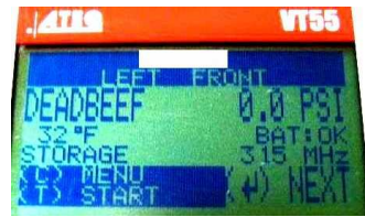
Figure 13: The TPMS trigger tool displays the spoofed packet with the sensor ID “DEADBEEF”. We crossed out the brand of TP sensors to avoid legal issues.
